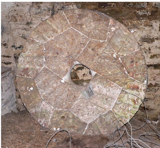
Fig. 13: French stone at Cawsey Meethe Mill, north Devon, made up from 14 individual blocks or burrs.
