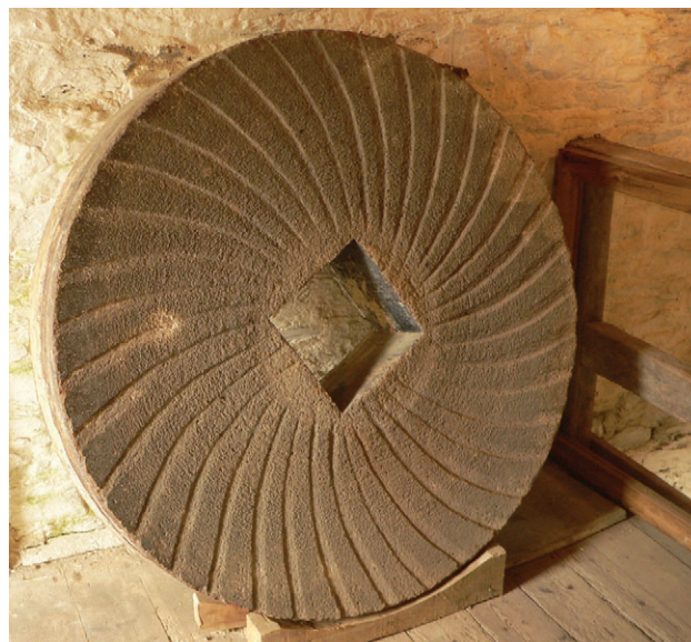
Fig. 14: Composition millstone with typical curved furrow dressing at Cotehele Mill, east Cornwall.
