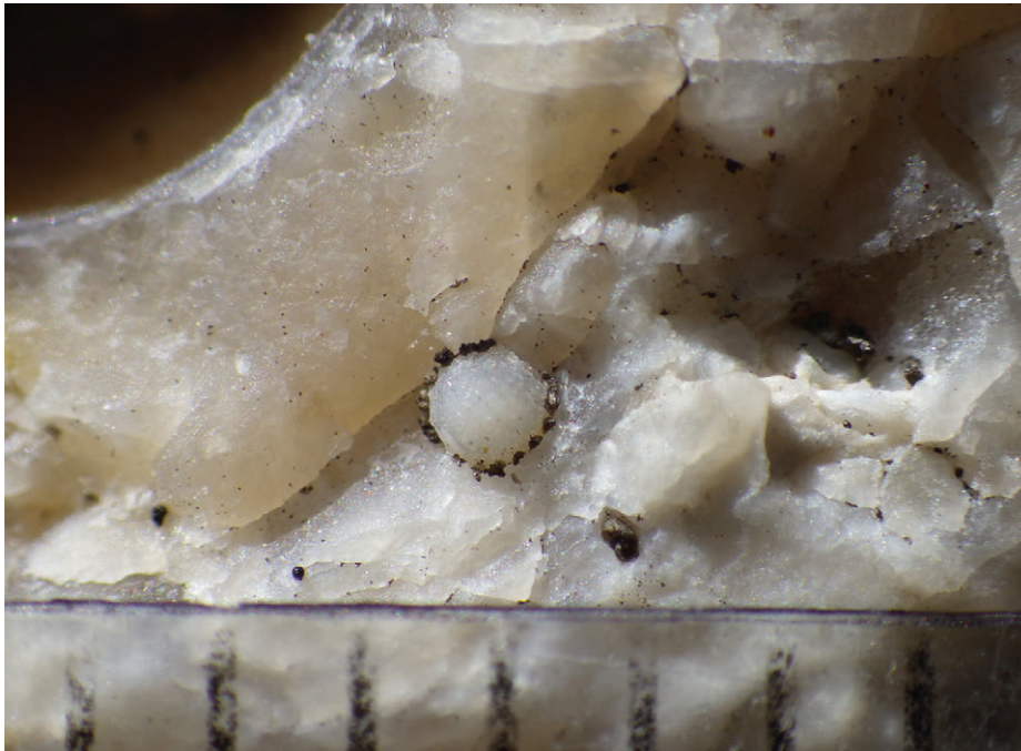
Fig. 5: Field photo of millstone at War Eagle Mill showing charophyte gyrogonite Gyrogonia cf. G. medicaginula (center). Scale in 1-mm increments.
