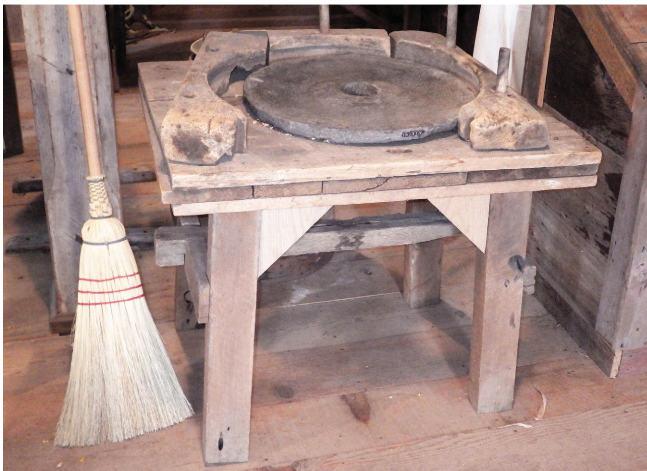
Fig. 8: Handmill (1952.37) inside Beckman Mill, Beckman Mill Park, Rock County, Wisconsin. Bedstone: 54.5 cm in diameter.
