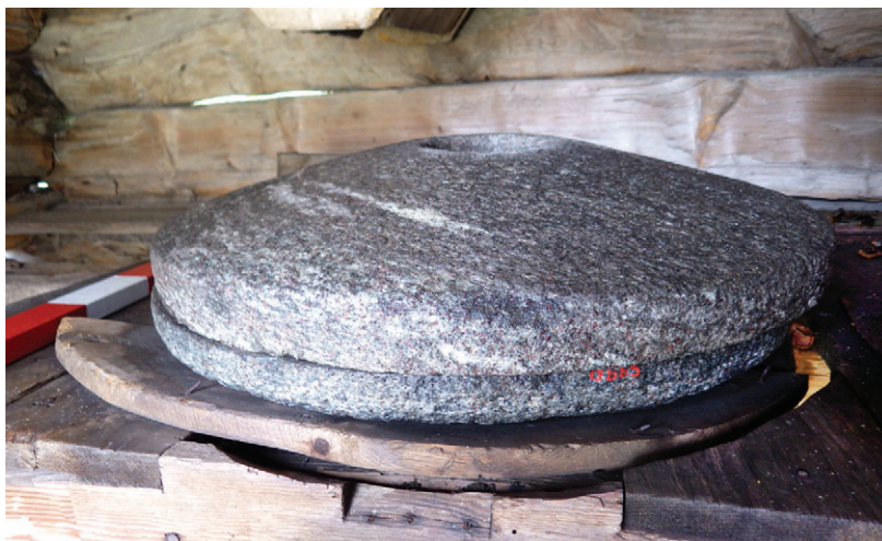
Fig. 4: Pair of muscovite mica-schist millstones (LC5990) inside Norsvin Mill. Scale is marked in 1-dm increments. The runner is laid directly on top of the bedstone.
