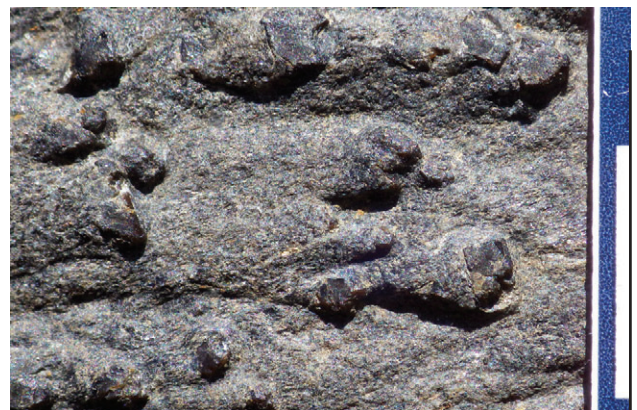
Fig. 13: Close-up of biotite mica-schist runner at Beckman Mill, showing staurolite porphyroblasts. Millstone is obliquely lit so as to show detail of flute-cast-like forms.
