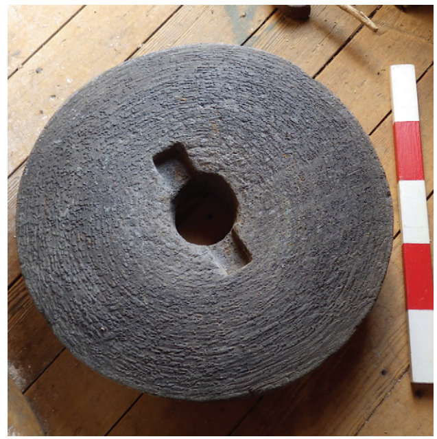
Fig. 11: Bottom of biotite mica-schist runner associated with a handmill in Beckman Mill (photographed inside Beckman Mill). The surface is obliquely lit to show distinctive circular wear pattern. Scale 50 cm.
