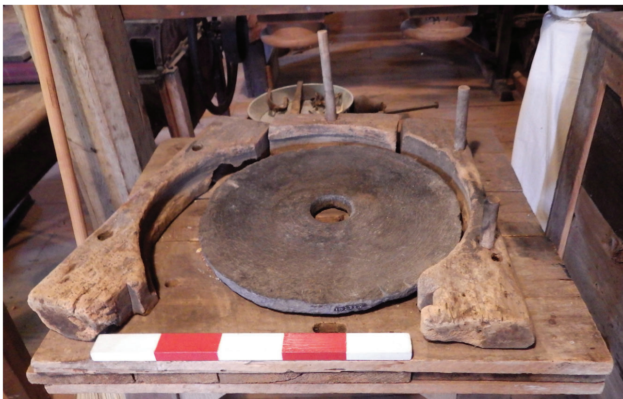
Fig. 9: Biotite mica-schist bedstone (1952.37B), surrounded by well-worn, presumed original housing. Scale 50 cm.
