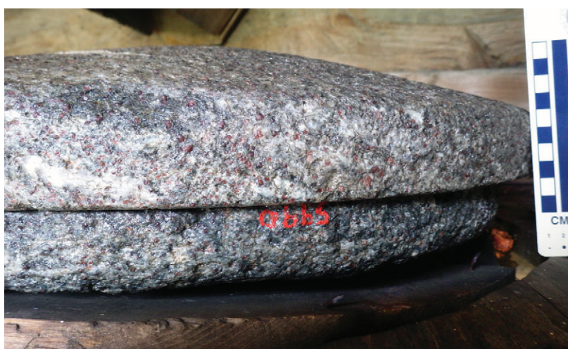
Fig. 5: Closer view of muscovite mica-schist millstones in Norsvin Mill. Scale and right side of millstones are foreshortened in the photo.
